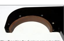
We will machine the aluminum arm and mold to contoured surfaces. This particular gripper is for holding reels during spin welding operation.
